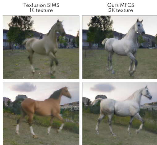
Figure 3. We show a comparison between Texfusion’s Sequential Interlaced Multi-view Sampler (SIMS, left ) [4] and our method ( right ) in accommodating high-resolution textures. Texfusion’s SIMS has rigid requirements on texture resolution and completely loses view consistency with a high-resolution texture. Our formulation of separating noise and color textures enables high texture resolutions without sacrificing view consistency.
