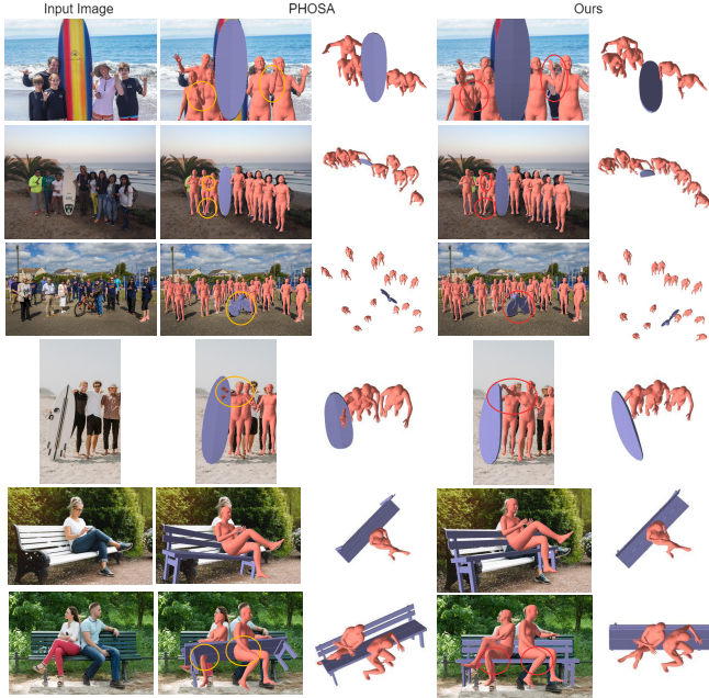
Figure 7. Our method, recovers plausible human-object and human-human spatial arrangements by explicitly reasoning about them. Here we demonstrate reconstruction on images with both humans and objects and compare PHOSA’s reconstructions to those produced by our method.
